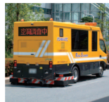
Radar survey for subsurface void detection
