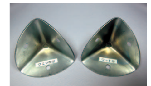
Left: Citric acid bath undercoat (little color irregularities) Right: Conventional bath undercoat (significant color irregularities)
