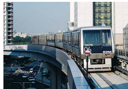
Yurikamome (Tokyo Waterfront New Transit Waterfront Line) This line was planned with the development of the Waterfront Sub-center, and in 1995, the section between Shimbashi and Ariake came into service as an automated guideway transit system. The line was extended from Ariake to Toyosu in 2006. It passes through the sightseeing spots of Odaiba and Rainbow Bridge, and connects central Tokyo and the waterfront sub-center. Source: Tokyo Metropolitan Government official photo archives.
