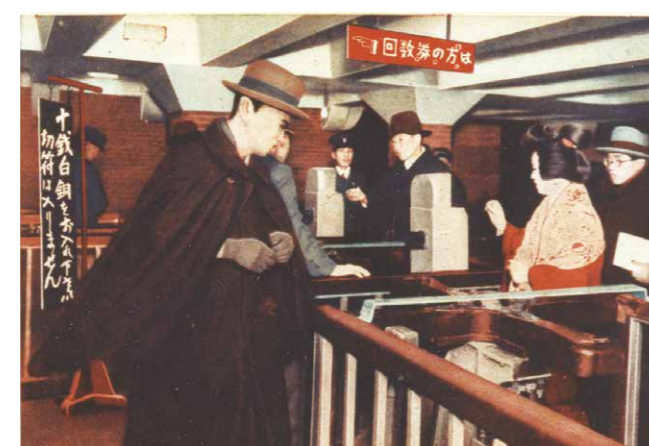
First ticket gates (Ginza Line) Turnstiles made in the United States were adopted to serve as ticket gates when service was launched. It was an innovative system at the time. Passengers dropped a ten-sen nickel coin into the fare collection box at the entrance to the turnstile and then pushed the cross-shaped wooden arm to enter. Source: Tokyo Metro Museum.
