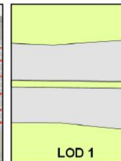
TransportationComplex provides surface geometry describing the actual shape of the object ■ TransportationComplex (Surface geometry) ■ Terrain surface
